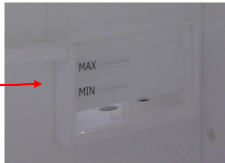
Figure 31: Water tank internal level indicators
