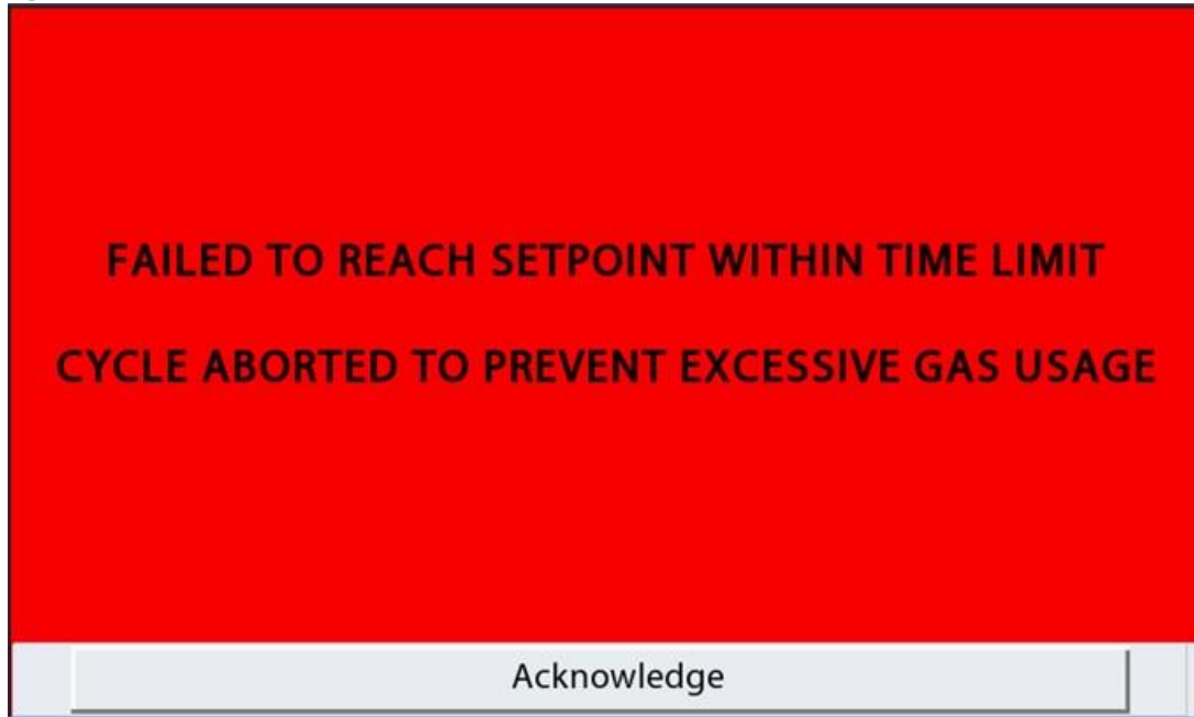
Figure 35: Failure to reach Set Point Alarm
