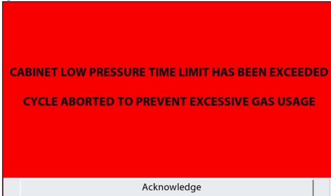
Figure 36: Low Pressure Time Limit Alarm
